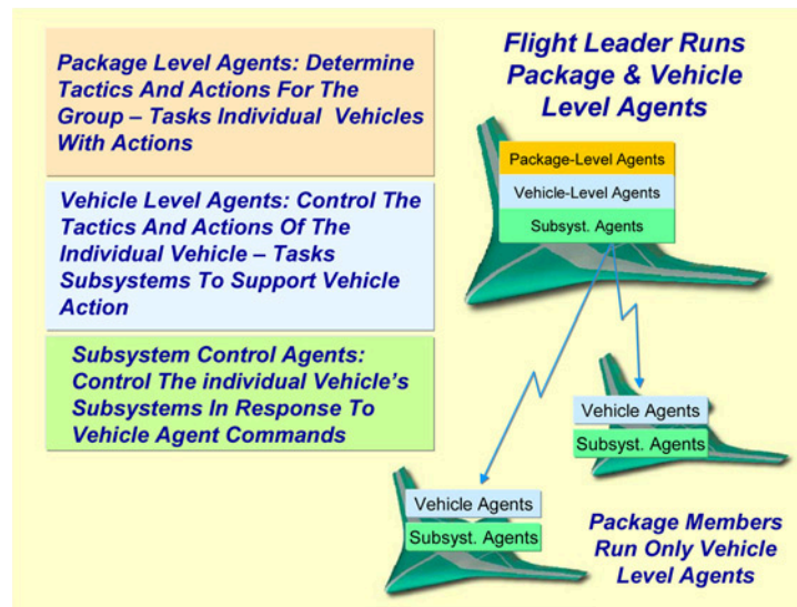
Fig. 3 ITAC multi-UAV C2 architecture.
